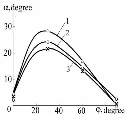
**Figure 4.** Dependence of the inclination angle of the crack trajectory on specimen orientation. As is seen, the character of the dependences presented for the mentioned states qualitatively is identical. The maximum deviation of the crack trajectory from the notch axis is held for
