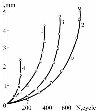
**Figure 2.** Kinetic curves of crack propagation.
