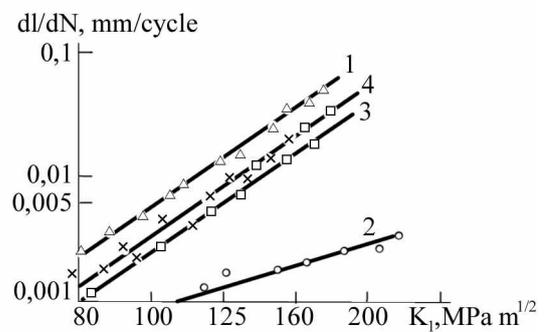
**Figure 3.** Dependences of the crack growth velocity on the value of the stress intensity factor.
