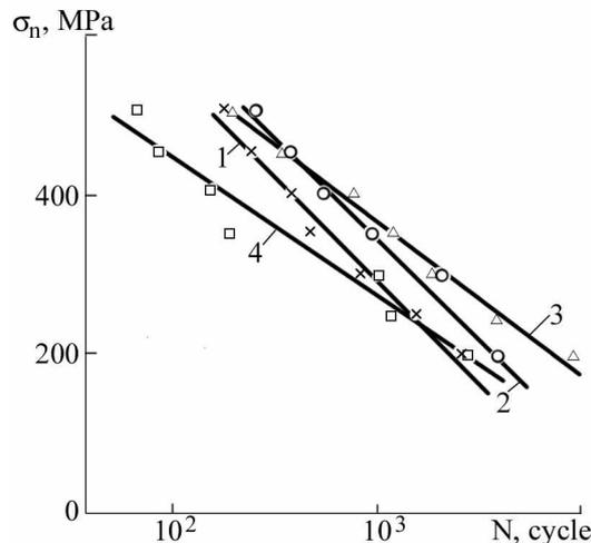
**Figure 1.** Dependences of the stress  $\sigma_n$  on the number of cycles  $N$  to fracture.
