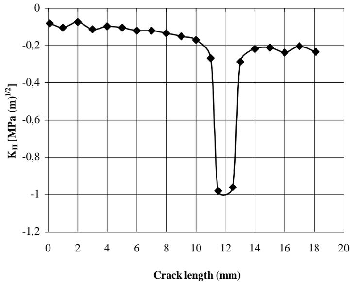
**Figure 10.** Variation of  $K_{II}$  with crack length for long crack
