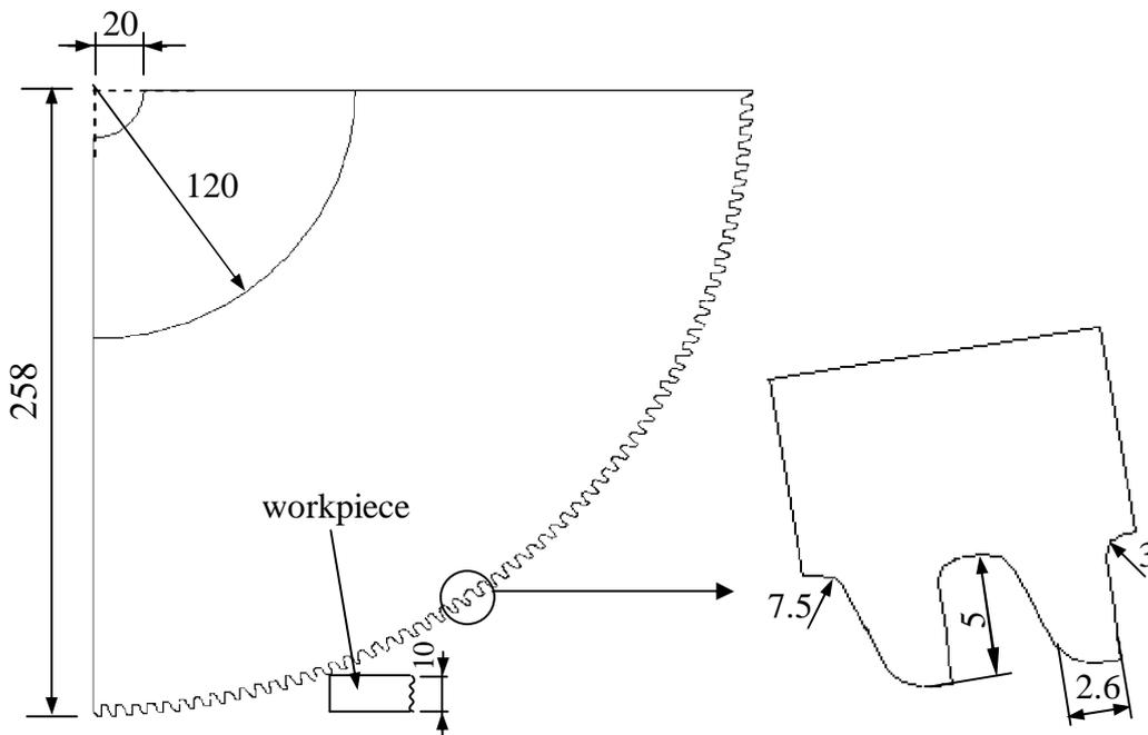
**Figure 2.** Geometrical model of the circular saw with a work piece and geometry of saw teeth.
