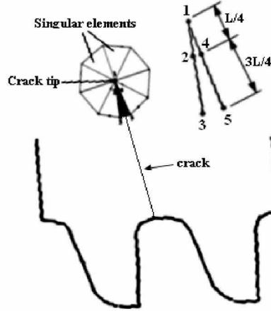
**Figure 5.** The location of the nodes used to calculate the stress intensity factor
