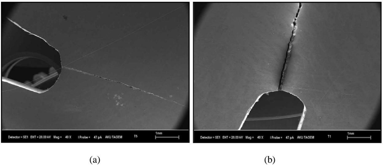
**Figure 8.** SEM photographs of the (a) small (b) large cracks
