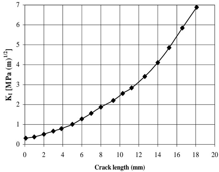
**Figure 9.** Variation of  $K_I$  with crack length for long crack
