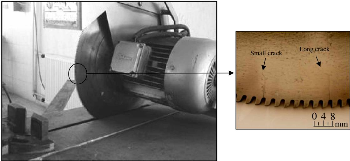
**Figure 1.** Conventional cutting machine and cracked circular saw
