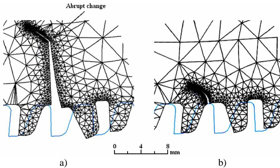
**Figure 11.** Finite element model of the cracks a) Long crack c) Small crack
