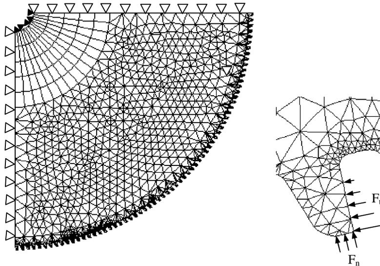
**Figure 4.** Finite element model of the circular saw, its boundary conditions and applied forces to teeth
