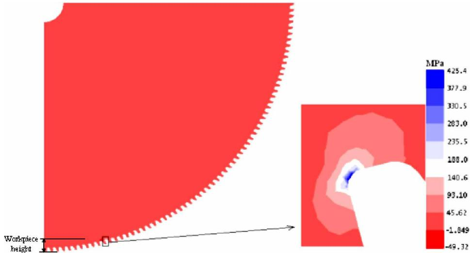
**Figure 6.** Principal stress distribution in the circular saw during the cutting process for 2880 rpm and 10mm dept of cut
