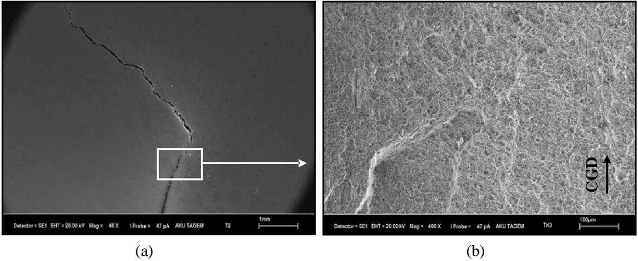
**Figure 7.** (a) Change of growing direction of the long crack, (b) Fracture surface of the circular saw
