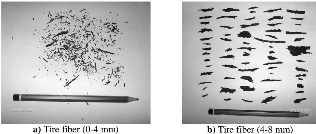
**Figure 1.** Waste tire fibers used in this study.
