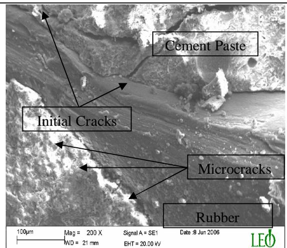
**Figure 6.** Scanning electron microscopy picture of rubberized concrete
