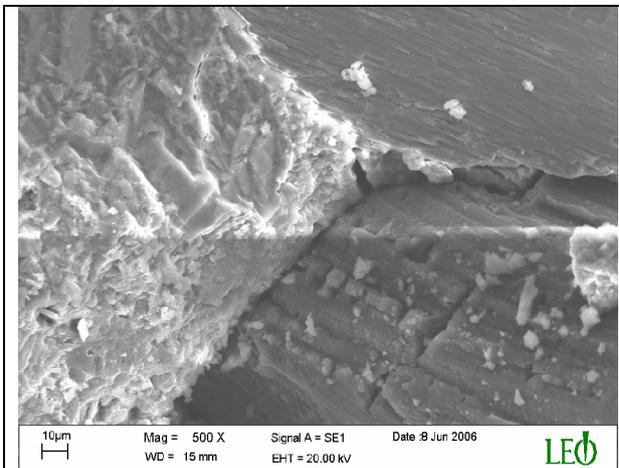
**Figure 5.** An image of ITZ between rubber tire, aggregate and cement paste
