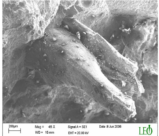
**Figure 4.** SEM image of pulled out rubber tire
