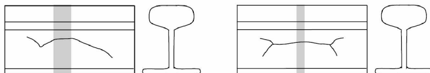
Figure 2. Horizontal split-web (HSW) fractures of weld zone [7].
